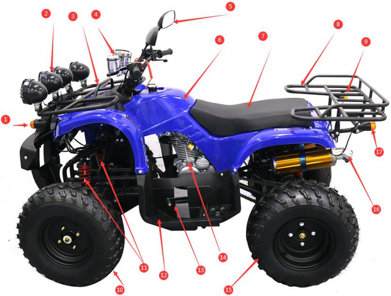
1. Front left turning light 2. Front Light 3. Front rack 4. Display 5. Mirror 6. Up plastic body 7. Seat 8. Rear rack 9. Rear right turning light 10. Front wheel 11. Front suspension 12. Bottom plastic 13. Foot shift 14. Engine 15. Rear wheel 16. Vent 17. Rear right turning light
