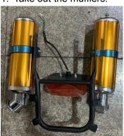
2. Unscrew the screws on the mufflers, install each muffler on the holder at the rear exhaust pipe as below.
