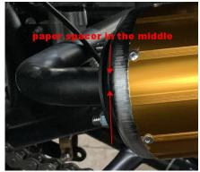
There is a paper spacer between the muffler and the holder when install, if the paper spacer was broken, replace
