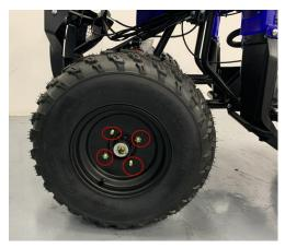
4th step: Install the rear tires (make the tread pattern and cycle valve outside).
